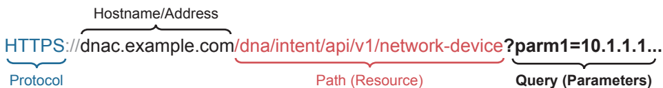
Figure 18-8 Example Components of a URI Used in a REST API Call
