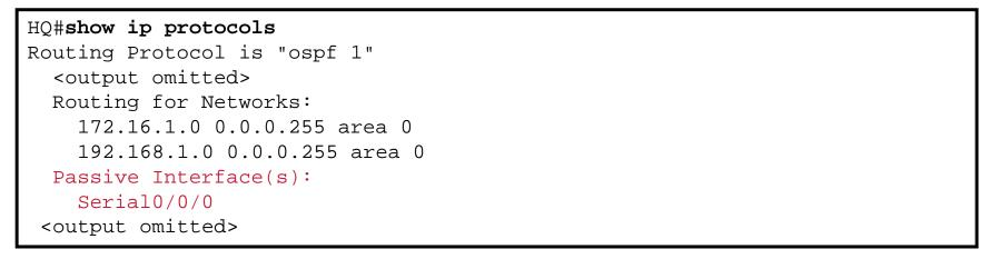
HQ has the interface toward the Branch router configured as passive. This is why the two routers are not forming an adjacency.
