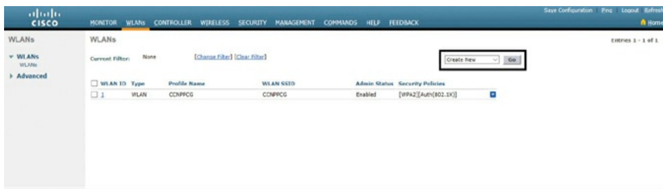
Figure 12-1 Creating a New WLAN
