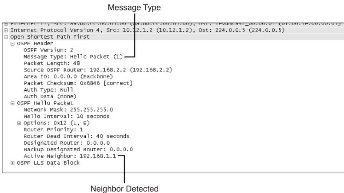
Figure 6-6 OSPF Hello Packet with Neighbors Detected
