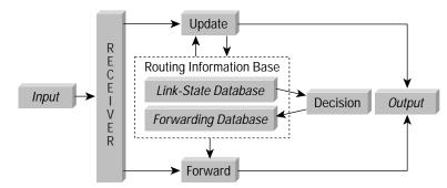
The *receive* process is the entry point for all data, including user data, error reports, routing information, and control packets. It passes user data and error reports to the forward process and passes routing information and control packets (hellos, LSPs, and sequence number packets) to the update process.
