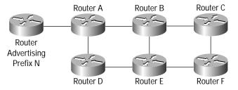
\Consider Figure 14 in the event of router B reloading. Router B would drop traffic if its neighbors include router B in their LSP while router B would not have a fully populated routing table. Thus router B would attract traffic but then not have enough information to be able to forward the traffic. This would result in packets being lost even though a valid alternate path (as used when router B is dead) exists.
