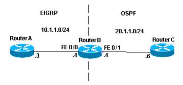
In this example, Router B has two Fast Ethernet interfaces. FastEthernet 0/0 is in network 10.1.1.0/24 and FastEthernet 0/1 is in network 20.1.1.0/24. Router B is running EIGRP with Router A, and OSPF with Router C. Router B is mutually redistributing between the EIGRP and OSPF processes. This is the pertinent configuration information for Router B:
