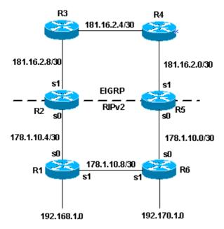
Using the topology as above, another method, which is sometimes more preferable, to avoid redistribution problems can be demonstrated. This method uses route—maps to set tags for various routes. Routing processes can then redistribute based on the tags. Note that redistribution based on tags do not work with RIP version 1 or IGRP.
