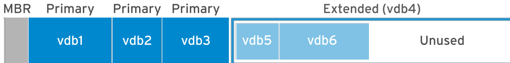
Figure 5.1: MBR partitioning of the /dev/vdb storage device
